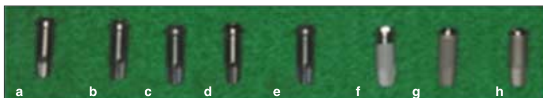
Fig. 1. Eight fixtures with differently treated implant surface. From left; a. Machined surface, b. 20 nm TiO 2 coated surface, c. CaP coated surface, d. Heat treated 80 nm TiO 2 coated surface, e. Heat treated CaP coated surface, f. Resorbable blast media (RBM) surface, g. Sandblast and acid-etched (SAE) surface, h. Anodized RBM surface.
